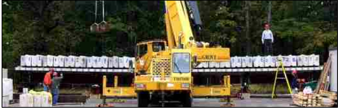
Figure 2.3: Straight concrete-filled rectangular steel tube TFG test specimen with concrete deck and loading blocks during testing (Sause, 2012)
