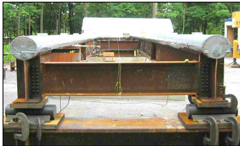
Figure 2.4: Straight TFGs with concrete-filled round steel tube top flange (Kim and Sause, 2005a, b)
