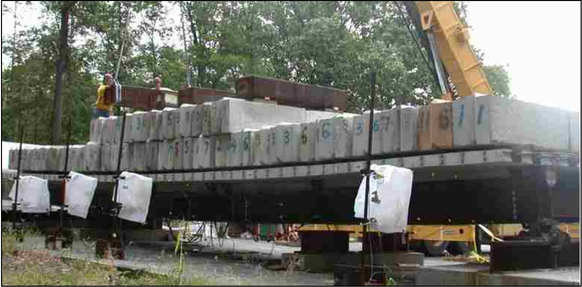
Figure 2.5: Straight concrete-filled round steel tube TFG test specimen with concrete deck and loading blocks during testing (Kim, 2005)
